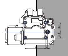
The positioner operates on the force-balance principle by comparing standard signal transmitted from a controller device with the angular rotation on the stem which conveys a positioning amplified pressure to the valve actuator.
