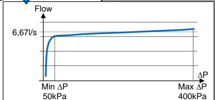
It is possible to preset the valve by acting on the mechanical stop of the actuator:
