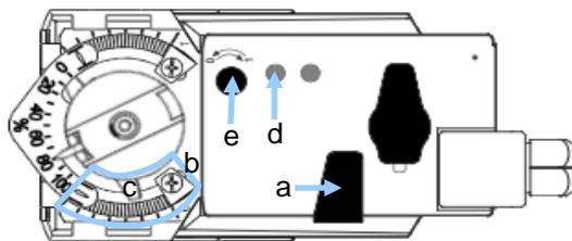
At the end of the auto stroke detection, the new maximum opening position is assigned to the opening signal, and the actuator will then redistribute the correspondence between the 0-10V signal and the opening position of the valve.
