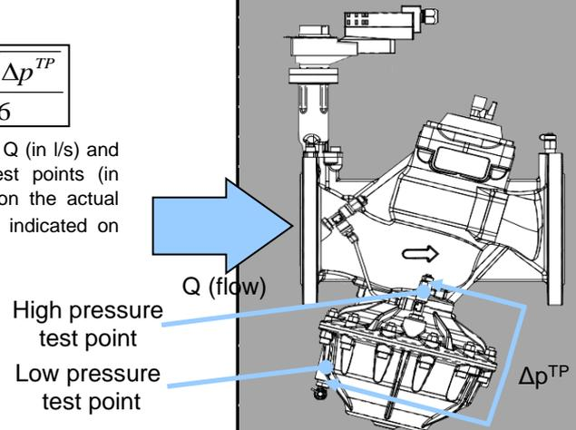
Valve presetting must be done according to the indications in the "Presetting" paragraph, Flow measurement indications are provided only as a check tool in case of problems on the system/valve.
