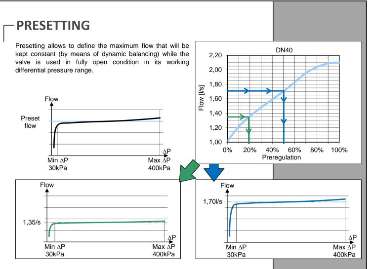
The flow regulating group has the authority on all its full linear stroke (full stroke modulation). By using a modulating actuator, this allows to maintain proportionality between the control signal and the actual output flow.
