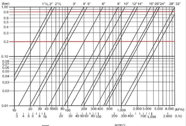
$Q_1 = flow rate [m3/h]$ m<sub>1</sub>= volumic weight [kg/dm3]  $\triangle p$  = pressure loss [bar]
