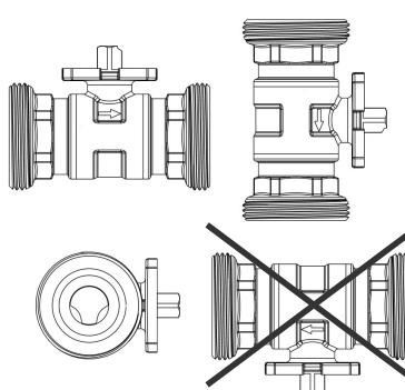
*It is important to install the valves so that the flow directions match the direction of the arrows indicated on their body. In order to obtain the best flowrate regulation the valves should be installed:*
