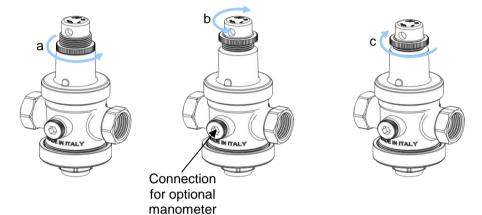
The pressure set with above procedure will be kept while the system is shut-off. Water flowing through the pressure reducer generates a headloss that will be deducted by the preset value.
