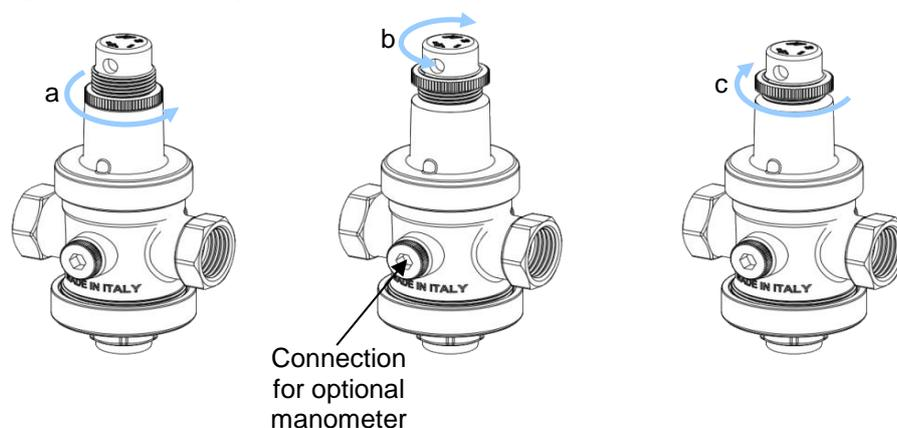
The pressure set with above procedure will be kept while the system is shut-off. Water flowing through the pressure reducer generates a headloss that will be deducted by the preset value.
