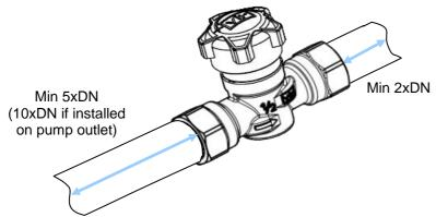
It is possible, at any time and even after the installation of the valve onto the line, to install onto the VIR 9522 valves a linear Vaurien actuator (for more information please refer to its specific technical sheet).
