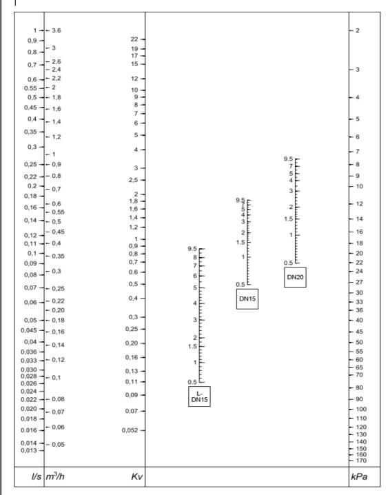
By using diagram above is possible to evaluate the presetting position of the valve with given design flowrate and headloss:
