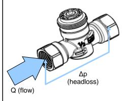
Formula linking flow Q (in l/s) and theoretical valve headloss  $\Delta p$  (in kPa).
