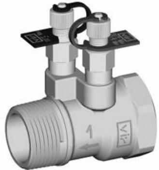
*VIR 9400 series metering stations allow to evaluate the flow passing through the branch of the circuit in which they are installed by measuring the differential pressure between their test points.*
