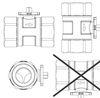
*It is important to install the valves so that the flow directions match the direction of the arrows indicated on their body. In order to obtain the best flowrate regulation the valves should be installed:*
